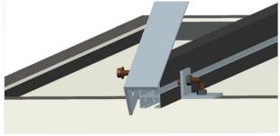
5, Insert the nut into the groove of the rail, and fasten the bolt to attach the bottom beam to the rail. (Notice: there are eleven holes in the bottom beam, choose hole 10 to insert the bolt. Please check the last page.)
