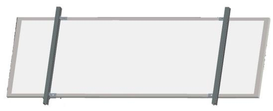
4, Fasten another bottom clip on the other side of the rail. Repeat the above steps to attach the other rail to the solar panel.
