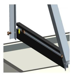
7, Insert a bolt into the tilt leg and though a gasket on the other side before screwing in the nut.
